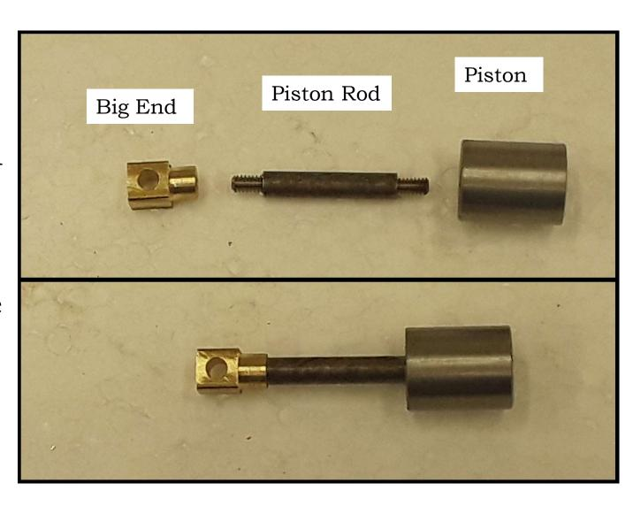
Piston Rod is 1/8" diameter Brass or Steel. Drill and tap with #2 x 56
