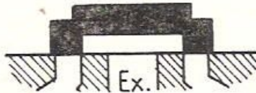
VALVE WITH SMALL LAP.
